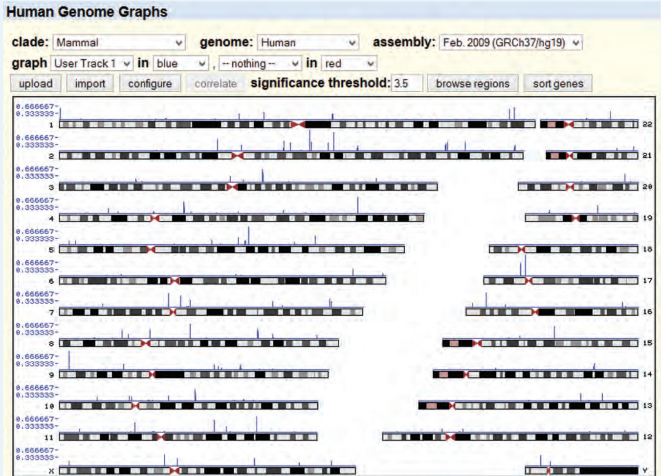
FIGURE 20.23 The UCSC Genome Graphs tool allows you to plot any UCSC or custom-selected tracks on ideograms. The distribution of NumtS genes is shown, that is, nuclear genes of mitochondrial origin.
